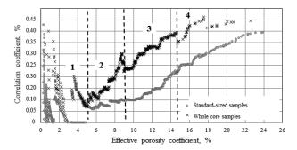
Fig. 2. Correlation coefficient plotted against porosity
