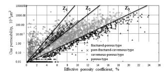
**Fig. 3.** Gas permeability plotted against porosity for samples divided by reservoir type
