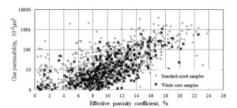
**Fig. 1.** The dependence of gas permeability on porosity
