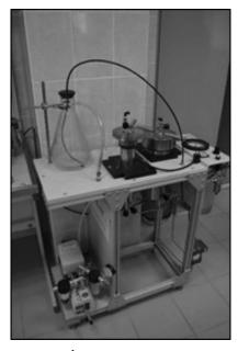
Fig. 2. MS-535 manual saturator
