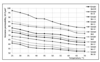
**Fig. 4.** Graph of variance of the permeability of core samples depending on the temperature in reservoir conditions
