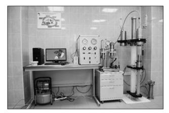
Fig. 3. UIP-ATM.002 training and research permeameter
