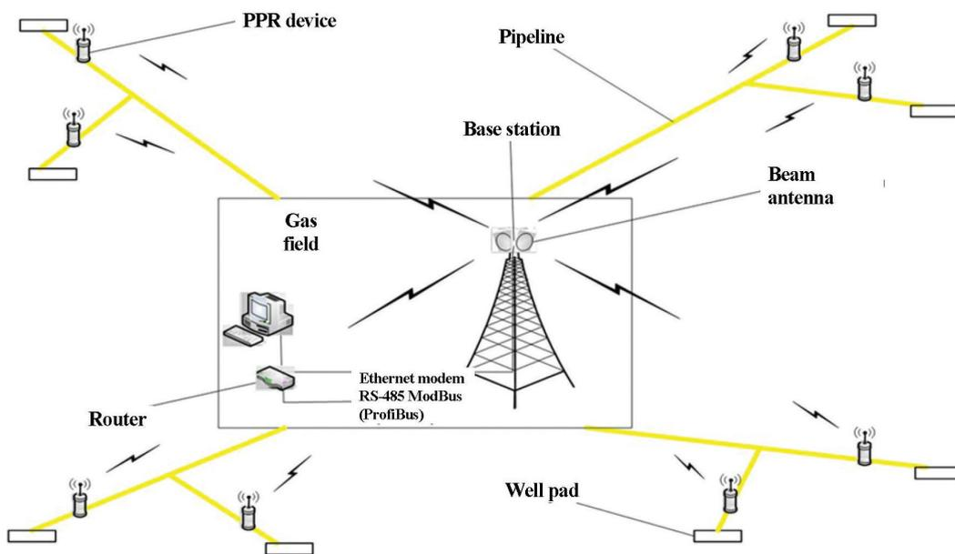
Fig. 1. Functional diagram of process parameters monitoring system
