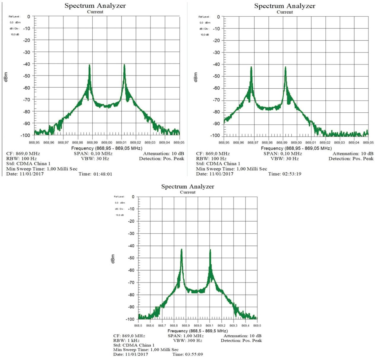
Fig. 3. Quartz resonator thermal chamber test results
