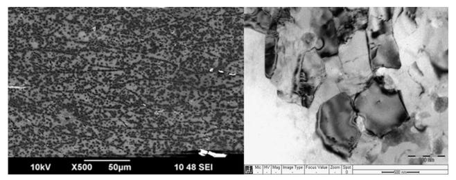
**Fig. 2.** Structure of alloy 1420: a) macrostructure of original sample; b) alloy's microstructure after ECAP severe plastic deformation
