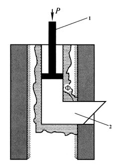
**Fig. 1.** Diagram of equal channel angular pressing: 1) piston, 2) pipe strip
