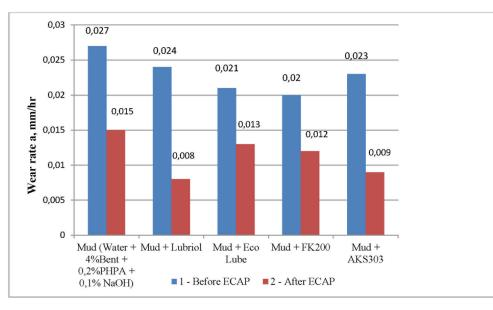
**Fig. 3.** Wear rate for alloy 1420 samples with coarse grain and SMC structure at T=293 K in drill fluid with different lubricating additives (confidence intervals established at 80% probability). (These results were obtained on friction machine UMT-2168)
